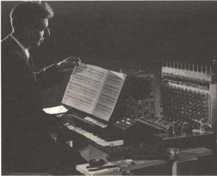
Hugh Le Caine demonstrating the prototype Touch-Sensitive Organ in 1954 (NRC photo)
